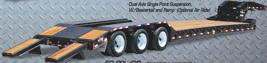
50 GSL/BR • CAPACITY: 100,000 lbs. 50 Ton Detachable Gooseneck, Three Axle Air Ride, W/Beavertail and Ramp
