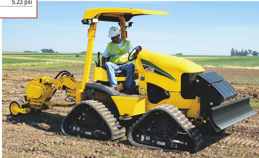
The quad-track Vermeer RTX750 features a one-piece automotive-style hood, which maximizes visibility during backfilling and transport.
